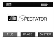
On the start up screen, you can use the buttons  $\blacktriangleleft$  or  $\blacktriangleright$  to select one of the three modes; FILE, IMAGE or SYSTEM mode. To confirm press the  $\Box$  button. The selected mode is highlight ed in red.
